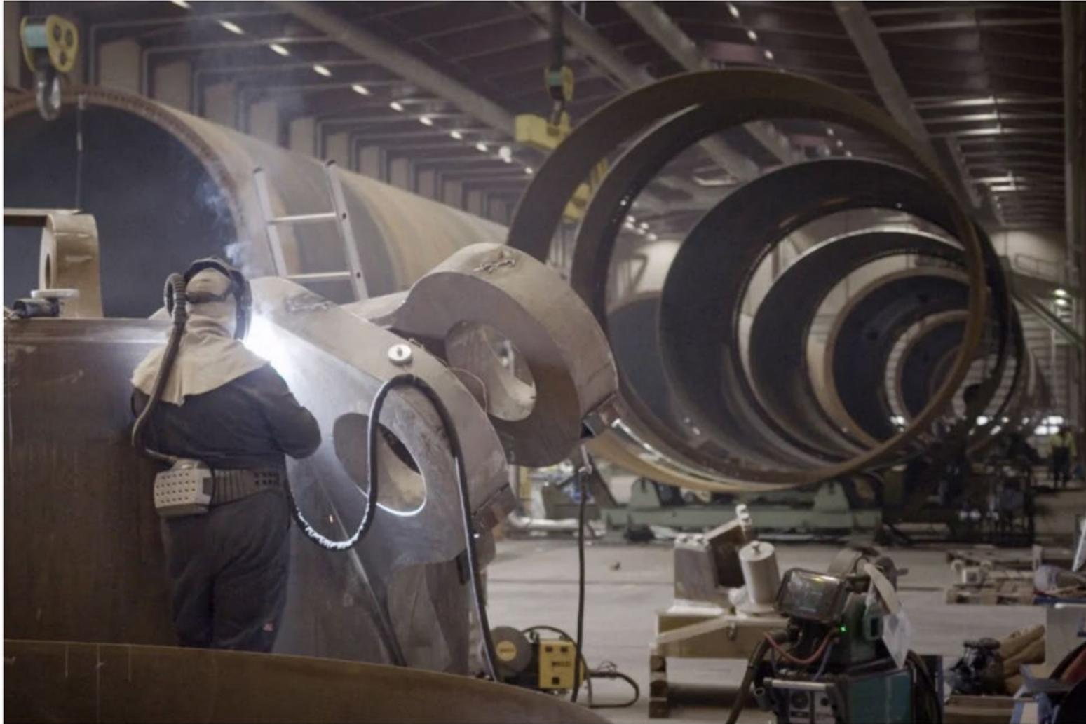
The components for the Tetra foundations were manufactured by Welcon A/S in Give, Denmark. Welcon is the world's leading supplier of offshore wind turbine towers, and its automated production lines are ideally suited for the manufacturing of the tubular braces and tanks for the Tetra concept. Photo credit: The TetraSpar Demonstrator Project ApS
